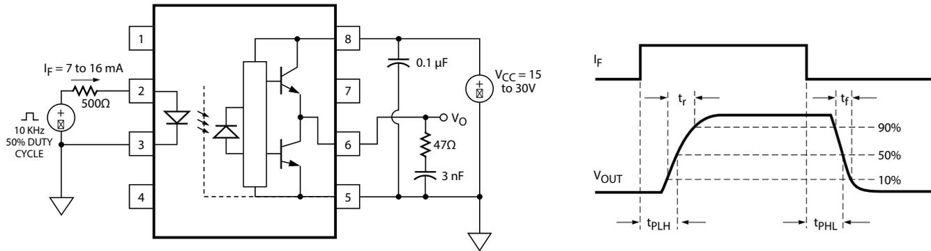
Figure 20: CMR Test Circuit and Waveforms
