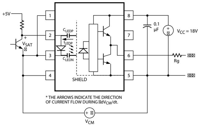
**Figure 26: Not Recommended Open Collector Drive Circuit**
