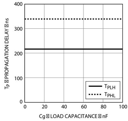
**Figure 17: Transfer Characteristics**
