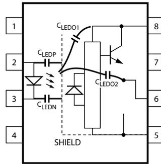
**Figure 25: Equivalent Circuit for Figure 19 During Common Mode Transient**
